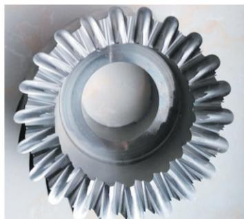
等前角圆弧齿刚齿刀具
