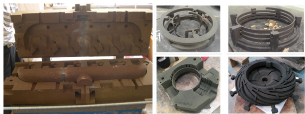
图12 3D打印整体打印复杂内腔型芯
