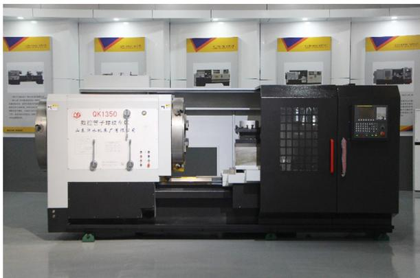
QK1350数控管螺纹车床
